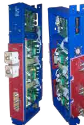
ATS Power Module (front and back with side panel removed)
