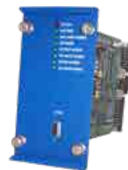
ATS Control Card Assembly
